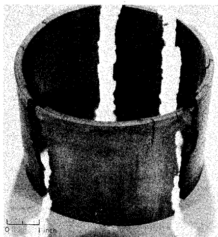
Fig. 1c Failure of plastic shell by rebound cracking.
